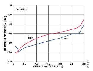
Figure 10. Harmonic Distortion (HD2, HD3) vs. Output Voltage for the High Current Driver—See Figure 54
