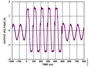
Figure 47. Overdrive Recovery of the VGA/Preamplifier—Gain Code = 1011
