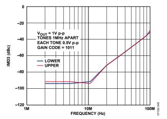
Figure 40. Third-Order Intermodulation Distortion (IMD3) vs. Frequency for the VGA/Preamplifier
