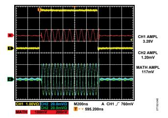
Figure 46. Gain Response for the VGA/Preamplifier, Yellow: Gain Code Select, Red: VGA Differential Output, Blue/Green: VGAP and VGAN
