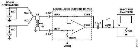
Figure 55. Test Circuit for IMD3 and OIP3 of the High Current Driver
