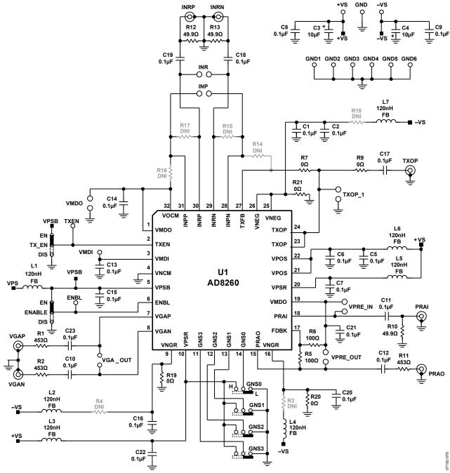
Figure 70. AD8260 Evaluation Board—Schematic Diagram
