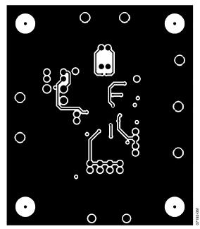
Figure 73. AD8260-EVALZ Secondary Side Copper
