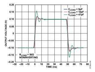
Figure 18. Small-Signal Pulse Response of the High Current Driver for Various Values of Load Capacitance,  $C_{LOAD}$ , and 50  $\Omega$  Load—See Figure 56
