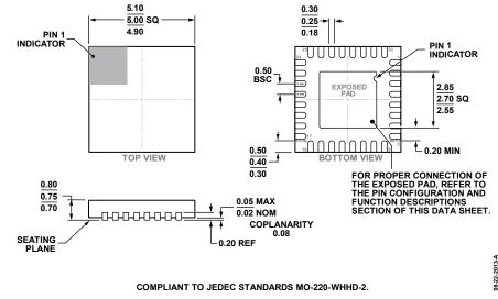
Figure 77. 32-Lead Lead Frame Chip Scale Package [LFCSP] 5 mm × 5 mm Body and 0.75 mm Package Height (CP-32-21) Dimensions shown in millimeters
