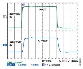
Figure 44. Large-Signal Pulse Response for the VGA/Preamplifier
