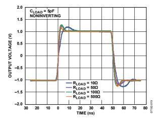
Figure 19. Large-Signal Pulse Response of the High Current Driver for Various Values of Load Resistance,  $R_{\text{LOAD}}$ —See Figure 56
