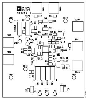
Figure 71. AD8260-EVALZ Component Side Assembly
