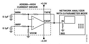
Figure 53. Test Circuit for Output Impedance of the High Current Driver
