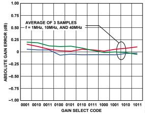
Figure 24. Absolute Gain Error vs. Gain Select Code for Three Samples for the VGA/Preamplifier at Three Frequencies Normalized to 1 MHz and Code 0110 See Figure 57
