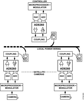
Figure 65. AD8260 Transceiver Application
