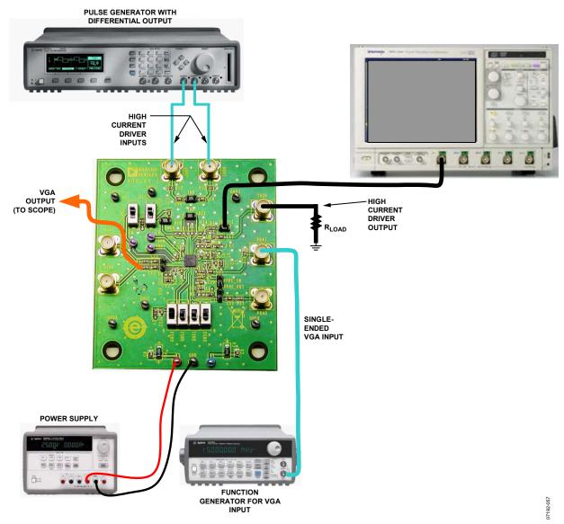
Figure 69. Typical Evaluation Board Connections
