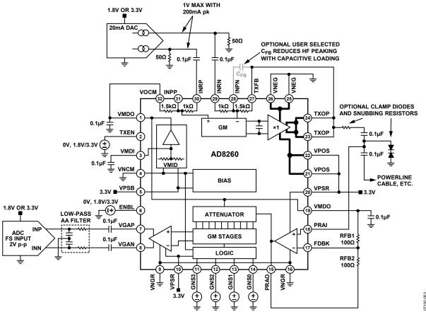
Figure 64. Block Diagram and Basic Application Connections
