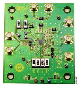
Figure 67. Top View of the AD8260-EVALZ
