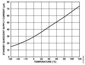
Figure 50. Standby Quiescent Supply Current vs. Temperature
