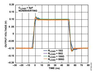
Figure 16. Small-Signal Pulse Response of the High Current Driver for Various Values of Load Resistance,  $R_{\text{LOAD}}$ —See Figure 56
