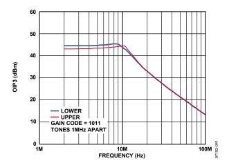
Figure 41. OIP3 vs. Frequency for the VGA/Preamplifier
