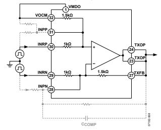
Figure 68. Gain-Setting Resistors of the High Current Driver
