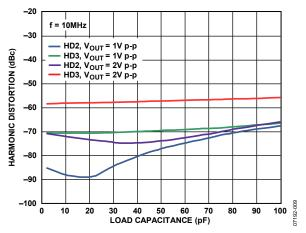
Figure 9. Harmonic Distortion (HD2, HD3) vs. Load Capacitance at Two Values of Output Voltage for the High Current Driver—See Figure 54
